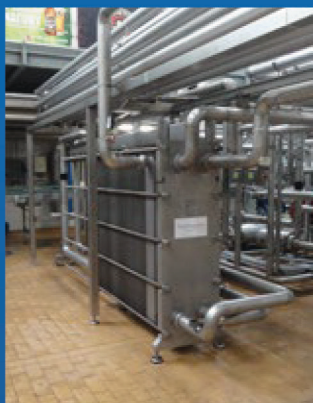
▲ A thermowave TL 500 FCGV unit, which boasts approx. 93 % heat recovery, is used as a pasteuriser for the high-temperature, short-time (HTST) flash pasteurisation of the beer for 15 to 30 seconds.
